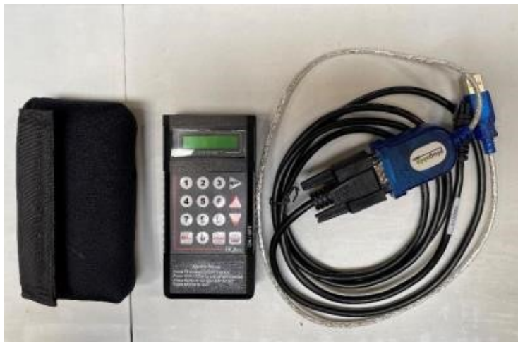
Figure 2.4: Data recorder device with pouch and connecting cable (CorTemp, HQ- FL, USA)
