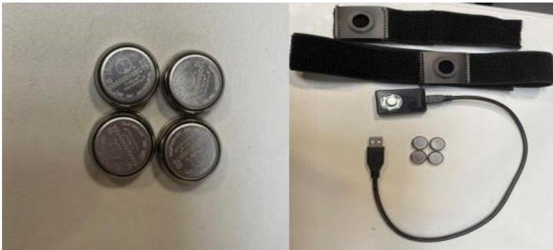
Figure 2.7: Thermocron Temperature Sensor Device; a) Thermocron iButton b) Custom fit Velcro belt with soft iButton Holder (top), data reader and cable (middle)
